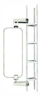
Designed to sample the relative phase relationship of radio frequency energy from 550-1600 kc antenna towers in directional antenna arrays, the Collins 564A-1 is made of two loops of #10 copper wire which may be connected either in series or in parallel. The wires are contained within a loop of 7/8" painted, copper tubing which serves as an electrostatic shield.
