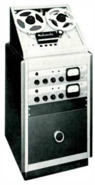
Input Impedance: High impedance unbalanced; 50, 250, 600 ohms balanced or unbalanced with plug-in transformers. Output Impedance: 600 ohms balanced with terminating switch to allow connections to high impedance input. Output Level: 0 VU. Power Requirements: Monophonic — Approx. 280 watts, 115 v, 60 cps (50 cps on special order). Stereo — Approx. 320 watts, 115 v, 60 cps. Size: Transport — 19" W, 15¾" H, 8" D. Amplifier — 19" W, 5¼" H, 8¼" D. Weight: Transport — 48 lbs. Amplifier — 12 lbs.
