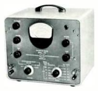
Ideal for FCC proof of performance tests and general laboratory use in measuring audio distortion, noise level and ac voltage level, the B & W 410 operates over a wider frequency range and provides increased sensitivity than earlier models.
