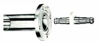
A very low VSWR line that is field proven for transmitter room interconnections, the Andrew 561 15/8" Teflon insulated line has compensated inner conductors. Anchor insulator connectors at each flange support the inner conductor on vertical runs and provide for differential expansion. Conductors and con-
