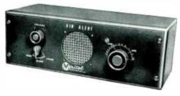
Designed to control visible and/or audible alarm circuits on CONELRAD signal from local or sky wave stations. Frequency tunable from 550 to 1600 kc. Built-in speaker operates upon alarm. Relay circuit is voltage regulated. External bell or light control terminals and antenna terminals on rear terminal board. Available for rack or table mounting.
