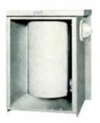
Coil provides isolation for the sampling line in directional arrays, presenting a high impedance for the line across the base insulator. Unit consists of a phenolic coil form which will accommodate 37 turns of RG8/U or similar solid dielectric sampling line. May be mounted on wall of tuning shack or in 49U-1 Housing (pictured). *Inductance*: Approx. 180 microhenrys. *Size*: 10" diameter, 18" L. *Weight*: 6 lbs.
