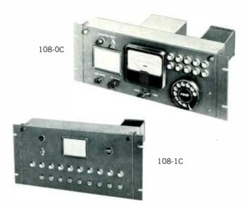
Power (each unit): 100-130 v, 50-60 cps, 25 va or less. Function Indication: By individual numbered pilot light indicators. Telephone Line: Two inexpensive signal circuit lines required; maximum dc loop resistance, 4,000 ohms. Size: 108-OC Control Unit—19" W, 7" H, 7½" D. 108-1C Transmitter Unit—19" W, 8¾" H, 7½" D.
