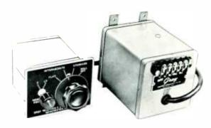
Normally used with standard microphone preamplifiers, making it unnecessary to purchase special audio input equipment when using magnetic cartridges. A convenient control permits instantaneous input switching from conventional records to microgroove. *Output Impedance*: 250 ohms balanced (150 or 50 ohms available). *Insertion Loss*: 20 db. *Output Level*: -67 VU at 4.7 cm/second. *Cable Length*: 18".
