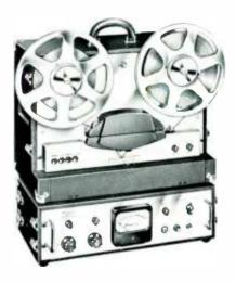
A portable recorder-amplifier combination, the M-90AC has a two-speed (7½ and 15 ips) direct tape drive with outboard capstan bearing assuring low flutter. Integrated design, torque motor supply and take-up tension achieve timing accuracy of better than 3 seconds in 30 minutes. Available without carrying case (M-90ACX) for rack mounting and in monoaural or stereo models. Also available on special order are remote control (M-90R) and console cabinet.
