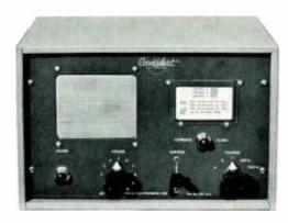
Designed expressly for CONELRAD Radio Alert. Built for 24-hour service, it gives automatic alarm with visual and aural warning. At time of radio alert, the speaker is automatically connected, you hear CONELRAD message and red pilot lamp on panel is lighted. Provision is also made for external alarm. Available in either cabinet or rack mounting models.
