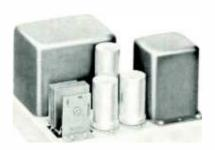
A plug-in module for Collins Consoles, this unit uses silicon rectifiers in the high voltage circuit for long life and to eliminate heat associated with vacuum tube rectifiers.
