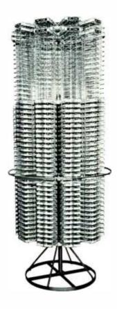
This sturdy, heavy Lazy Susan rack holds 500 of the Series 300 Collins automatic programming equipment tape cartridges. Ten chrome-plated racks with 50 slots each make storage and selection of cartridges fast and simple. Revolves easily on roller bearing hub and will not tip regardless of arrangement of cartridges. Cartridges held in wire holders at an angle to prevent slipping out while the rack is being revolved. Shipped knocked down. Size: Approx. 72" H, 36" diameter. Weight: Approx. 50 lbs.
