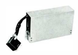
Used in Collins 212E-1 Console, this unit has four relays to control studio speakers and warning lights. Each relay is provided with a series shunt circuit to minimize switching transients and arcing. Noise is held to a minimum by mounting the relays on rubber. The 409X-2 Power Supply provides 12 v dc at 1 amp and studio wiring provides power for the warning lights.
