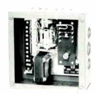
TOWER LIGHTING UNIT — Meets FCC requirements by metering lighting current to check bulbs and flasher. Latching relay allows overriding photocell control for Civil Defense purposes. Rated 20 amps ac (Type 108-5A-1).
