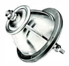
Designed to carry RF transmission line through a wall. Complete assembly includes heavy electrical glass feed-thru bowls, cork gasket and steel mounting flange with six 3/16" mounting holes. Bowl is 6-5/16" maximum diameter and 4 $\frac{3}{8}$ " high. Mounting flange has  $7\frac{3}{8}$ " diameter. Fittings include spun aluminum corona shield,  $\frac{1}{2}$ "-13 threaded stud (except 135-15-4 which has  $\frac{5}{8}$ "-18 threaded stud, hollow), washers and nuts
