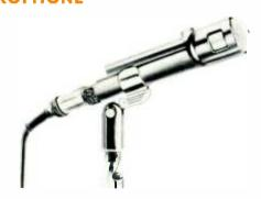
This microphone provides high discrimination against sounds from back hemisphere. Permits close talking with no bass accentuation and increases working distance over pressure microphones by factor of 1.7:1 due to polar pattern. Clamp-on stand mount with \(^{5}\_{8}"-27\) thread, \(^{1}\_{2}"\) pipe thread adapter and 20' cable included.
