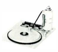
DC CURRENT UNIT - Installed in cathode circuits for indication of plate current. With positive thyrite disc overvoltage protector. Available in 300 ma (Type 108-9A-1), 600 ma (Type 108-9B-1), 1,200 ma (Type 108-9C-1) and 2,400 ma (Type 108-9D-1) ratings.
