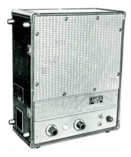
An ideal companion unit designed to match the Ampex 601 Series Recorder, the 620 has an 8-inch speaker that utilizes a high degree of bass and treble boost without undue harmonic or intermodulation distortion. The 10-watt power amplifier is of push-pull design. It is conventional high fidelity type but is unusual for its fast transient overload recovery.
