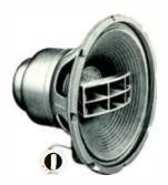
A coaxial, 12" speaker, the H-222 has electrically and acoustically independent "woofer" and "tweeter." and employs the through-bore compression driver tweeter. Frequency Range: 30-15,000 cps. Impedance: 16 ohms. Power Rating: 25 watts. Baffle Opening: 10½". Weight: 12 lbs. Jensen transformer (ZY-2003) for H-222 speaker matches to 600 ohms.
