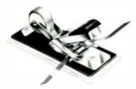
Used for magnetic recording tape, this unit cuts two rounded indentations in the tape splice, giving the splice a "Gibson Girl" shape and leaving the edges of the tape free of adhesive. The unit can be removed from its base and mounted directly on any tape recorder. It comes complete with a roll of splicing tape and tape feed.
