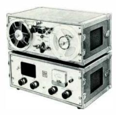
The PT6-6A Recorder and PT6-6J Amplifier are designed for either rack mounting or portable use. Powered by two-speed hysteresis synchronous motor for 7½ and 15 ips, selectable by switch. Low impedance and high impedance inputs are provided as well as 4, 8, 16 and 500 ohm outputs. The unit includes full-track erase and record/playback heads (half-track heads may be specified at no additional cost).
