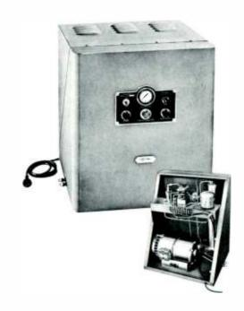
A piston type compressor unit that provides dry air for pressurization of air dielectric coaxial transmission line, the 1910A uses carbon rings to assure oil-free dry air and years of maintenance-free service. The compressor unit is driven by a heavy duty ½ hp motor.
