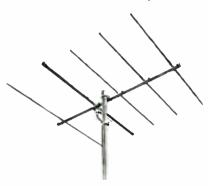
Average Gain: 9 db. Typical VSWR: Under 1.5. Typical Rear Signal Rejection: 25 db. Power Handling Capacity: 60 watts. Input Connector: Type AN-SO-239 (Amphenol Type 83-1R). Polarization: Horizontal or vertical.
